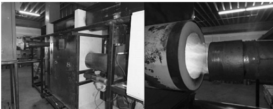
Figure 1. Pyrolysis system with combustion of pyrolysis vapors (Courtesy of Jerry Whitfield)
