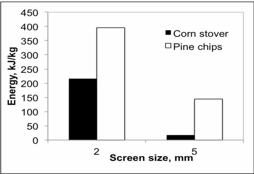
Figure 13. Energy consumption of grinding corn stover and pine chips by hammer mill. (Gil et al., 2008)
