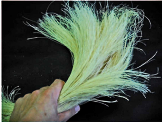
Figure 3. Group of mechanically extracted fibers diameter ranges between 90 and 250 \mu m (Osorio et al. 2010)
