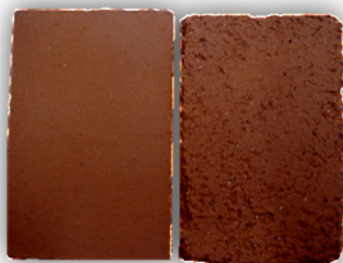
Figure 8: Bricks with clay alone (left) and with 10% of residue (right).
