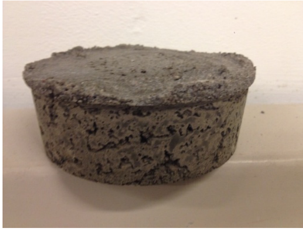
Figure 4: Set specimen added 1.8g SP.
