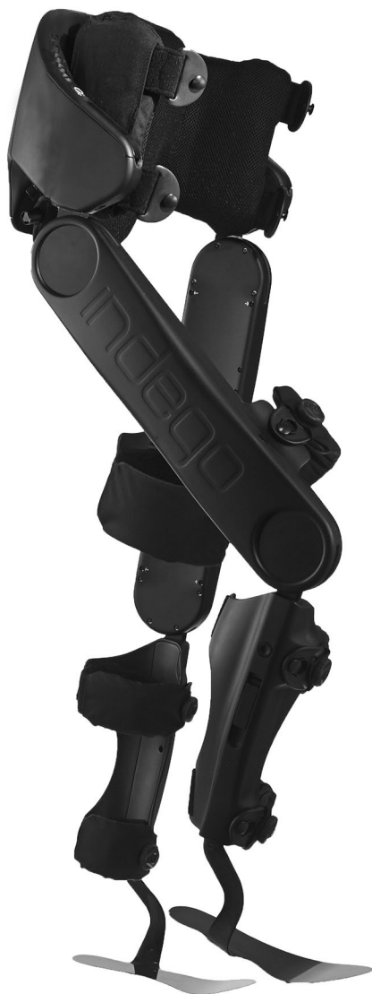
Fig. 13.4 The Indego is a lower extremity exoskeleton designed to enable individuals with lower extremity weakness or paralysis due to SCI and other conditions to stand, walk, and perform stand-to-sit transitions. (Courtesy of Parker Hannifin.)
