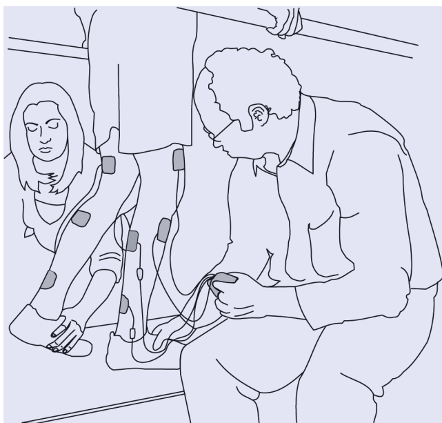
Fig. 12.1 Compex Motion functional electrical stimulation (FES) system for walking. The Compex Motion system has four stimulation channels that can be increased by connecting multiple stimulators in series. (Courtesy of Rehabilitation Engineering Laboratory (REL), Toronto Rehabilitation Institute—University Health Network, Canada.)
