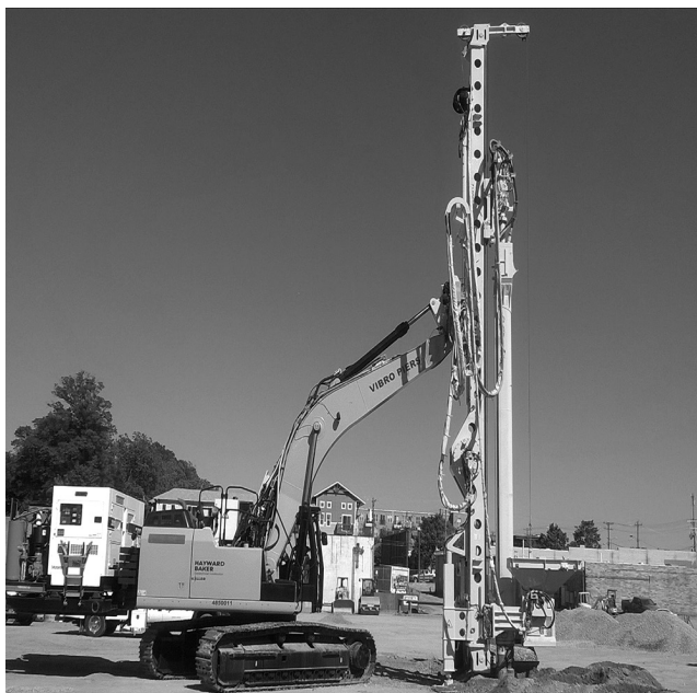
Figure 4.4 Attachment for standard excavators to carry out stone column installations. (Courtesy of Keller Group plc, London, UK.)
