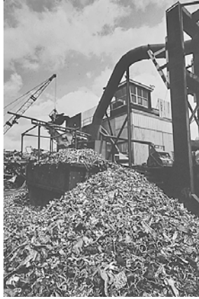
Pile of shredded aluminum in front of an automobile shredder, Jackson, MS, 1972. Photograph by Bill ShROUT for US Environmental Protection Agency (412-DA-3769). Courtesy National Archives
