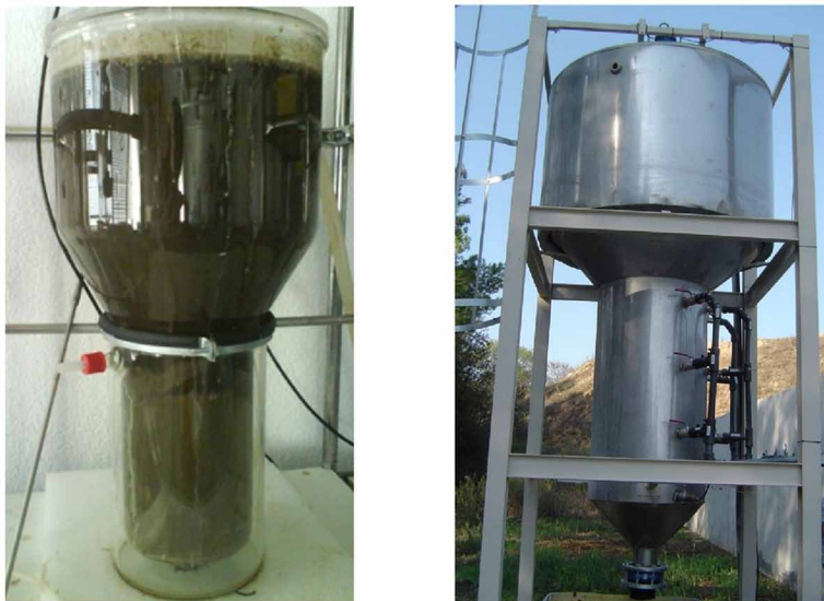
Figure 6. Lab scale struvite precipitation reactor (left), and pilot plant at SAT Sant Mer Biogas Plant (Vilademuls, Girona) (right)
