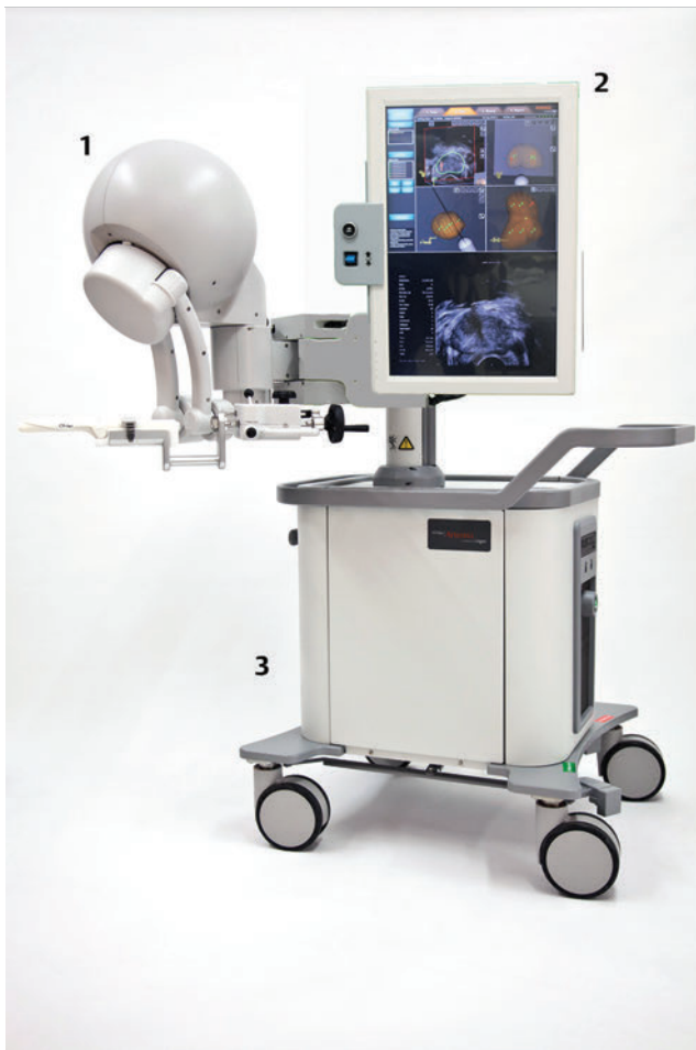
Fig. 9.5 Artemis (Eigen), one of the 5 fusion devices that are currently approved by the U.S. Food and Drug Administration. The device has three major components: (1) a mechanical robotic arm, which provides localization tracking; (2) a computer screen to visualize the fused images; and (3) a computer to perform the calculations involved in coregistering the uploaded MR images with freshly obtained TRUS images.
