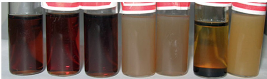
Fig. 7.33: Appearance of bio-oil emulsions from different species of biomass: rice husk, rice straw, rosewood, Mongolian Scots pine, bamboo, grassiness, and algae (from left to right).
