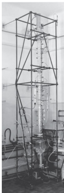
Fig. 9.16: Pilot-scale distillation column ( Illudest ) at the Faculty of Chemistry and Chemical Engineering, Babeş-Bolyai University of Cluj-Napoca, Romania. (Adapted after [20].)
