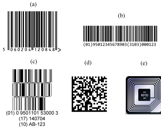
Figure 3. GS1 data carriers: (a) EAN/UPC barcode, (b) GS1-128 barcode, (c) DataBar, (d) DataMatrix, (e) RFID
