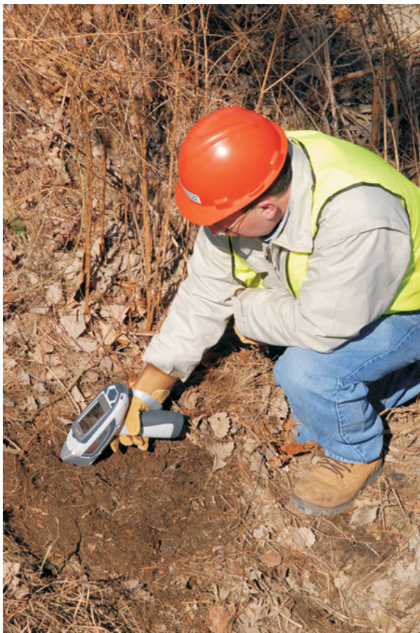
Figure 3. A portable XRF analyzer employed for soil testing. Reprinted with permission; copyright Thermo Fisher Scientific.
