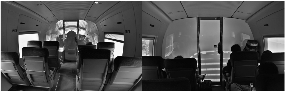
Fig. 17: An example of deactivated/activated switchable glazing
