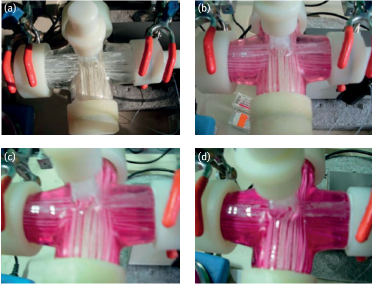
Fig. 5.8: Snapshots of a 40 cm 3 crossed-hollow fibers bioreactor under step-stimulus at: (a) 1 min; (b) 90 min; (c) 240 min; (d) 380 min. Williams' medium at flow rate of 1.5 ml/min is used as tracer.
