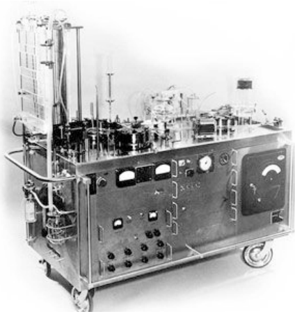
Fig. 3.21: Heart-lung machine used by John Gibbon successfully on an 18-year-old patient [45].
