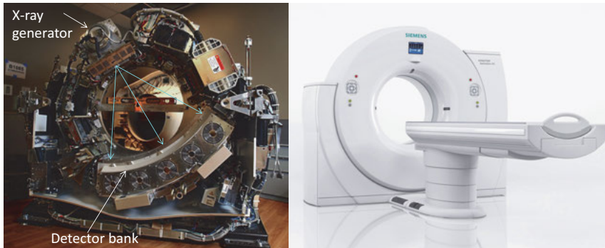
Fig. 5.30: CT unit without cover and with cover. X-ray generator and detector bank is housed inside behind the cover ( www.healthcare.siemens.com/computed-tomography/ ).
