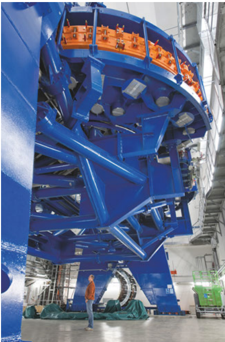
Fig. 10.12: Gantry for carbon ion radiation treatment at the Heidelberg Ion Beam Therapy Center is a 360° rotating beam delivery system. It weighs 670 tons, is 25 m long, and 13 m in diameter spanning three stories (photo reproduced from Heidelberg University Hospital https://www.klinikum.uni-heidelberg.de/Gantry,image-2012.129328.0.html ).
