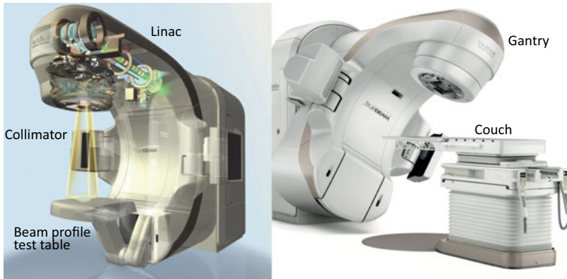
Fig. 9.1: Modern medical linac used for cancer treatment. The gantry housing a linac, collimators, and shutters circles around the patient at the center for irradiating tumors with high energy x-ray photons incident from different angles (courtesy Varian Medical Systems International AG, Switzerland; all rights reserved).
