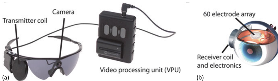
Fig. 15.21: Epiretinal implant of the Argus II type uses a camera incorporated in a pair of glasses. After processing the video images (VPU), they are sent wirelessly to a receiver implanted on the bulbus. From there the signal is transferred by wire to a micro-electrode array, tacked to the retina (reproduced from [27], © Creative Commons).
