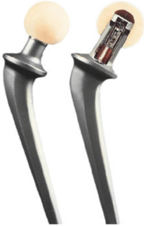
Fig. 15.11: Hip shaft with integrated strain sensors in the neck of the implant for measuring forces and torques during various activities (reproduced from [16] by permission of Elsevier Publishing Inc.).
