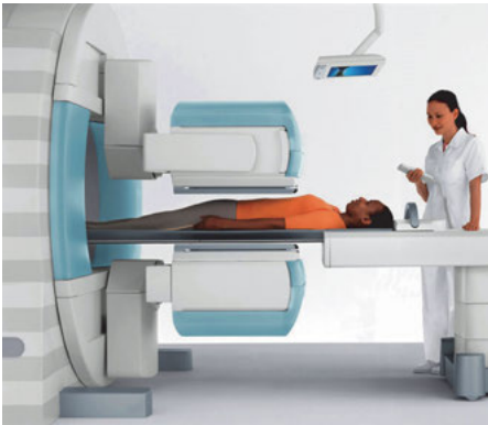
Fig. 6.9: SPECT Siemens Symbia SW06 with two opposing detector heads (reproduced from www.siemens.com/press ).
