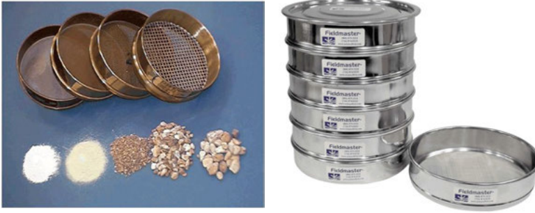
Figure 6.21: Series of stainless steel mesh screen sieves for soil or bottom-ash separation. (Left) The individual screens with retained particle fractions. (Right) The screen cascade.
