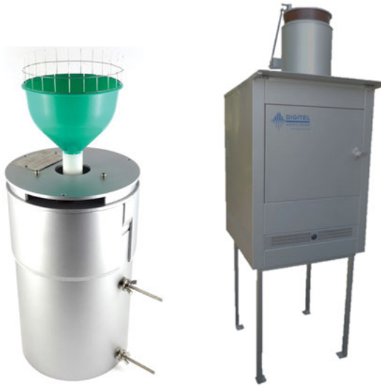
Figure 4.7: (Left) Rain bulk sampler for collecting rainwater and particulate matter. (Right) Wet-only rain water sampler with several polyethylene sampling bottles (to be switched motor-driven), motor-driven precipitation-controlled funnel lid, ambient temperature sensor and programmable climatization (heating/cooling).
