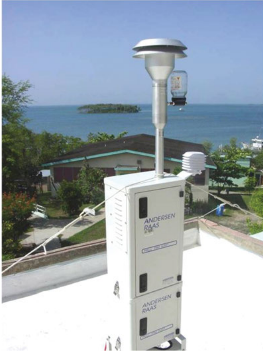
Figure 4.26: Photography of a high-volume aerosol collector unit with circular sampling head. Reproduced with permission from Roy A. Armstrong, Ph.D., Bio-optical Oceanography Laboratory, University of Puerto Rico.
