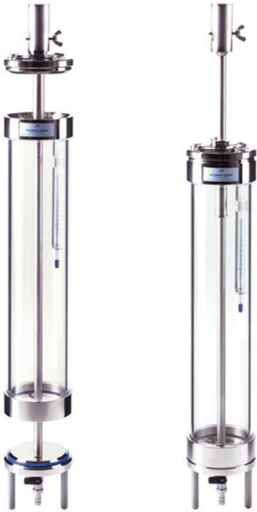
Figure 4.8: Ruttner sampler (left: open, right: closed) for collecting water from different depths suitable for taking samples in lakes, sea, water borings, wells and so on. Sampler volumes cover a range of about 1–5 L.
