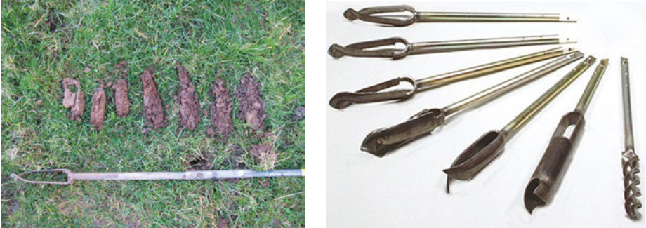
Figure 4.11: (Left) Soil samples from different depths by using a hand-driven soil auger. (Right) Different soil auger types specifically used depending on the soil conditions (e.g., hardness, dryness, texture).
