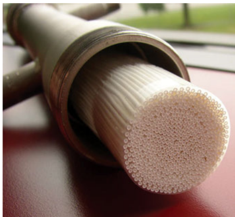
Figure 6.27: Hollow fiber bundle for high-efficiency cleaning of water.
