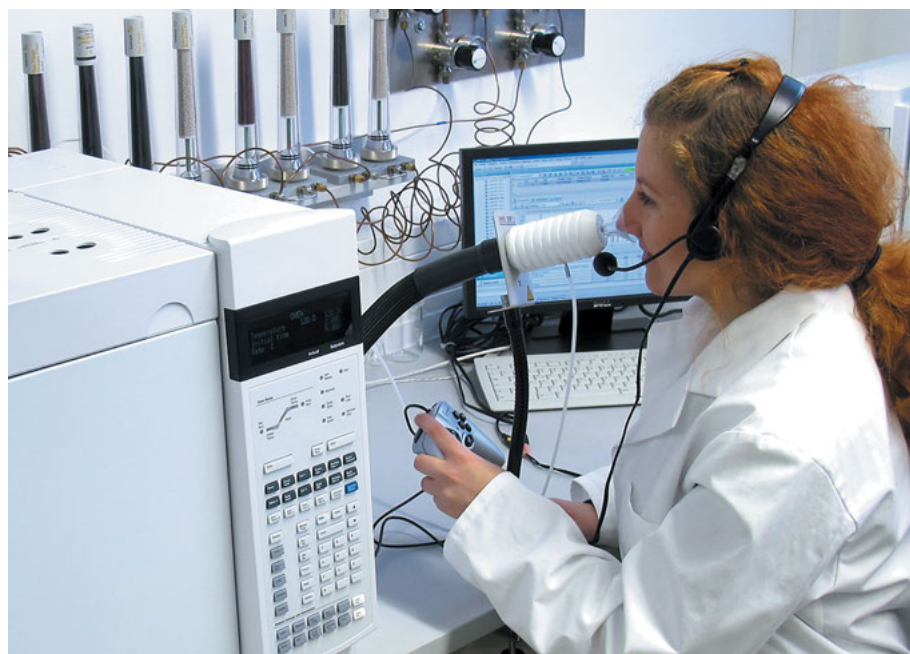
Figure 7.59: Sniffing person acting as detector. Reproduced with permission from Fraunhofer WKI / Manuela Lingnau.
