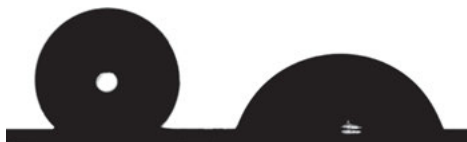
Fig. 6.3: Wetting transitions observed under vibration of a 15- \mu\text{L} water drop deposited on a micrometrically rough polydimethylsiloxane surface. (Left) Initial Cassie state. (Right) Cassie impregnating state induced by vibrations [25].
