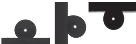
Fig. 11.20: A 10- \mu L droplet deposited on a surface built of lycopodium particles (for details, see Reference 73).
