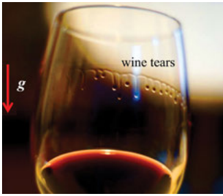
Fig. 7.1: The effect of wine tears. Wine is climbing upward against gravity \vec{g} .
