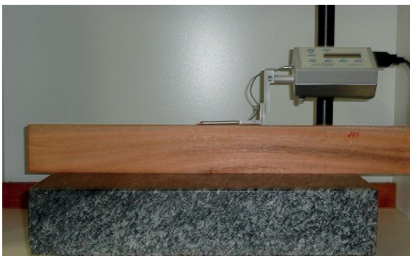
Fig. 7.12: Methodology for roughness measurement on wood surfaces.
