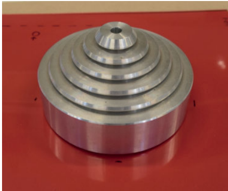
Fig. 1.11: Apparatus for the dry heat test.
