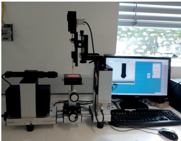
Fig. 1.4: Contact Angle System Dataphysics OCA 20.
