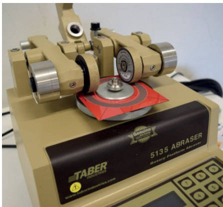
Fig. 1.6: The TABER® rotary platform abrasion tester – Model 5135 – taber abramer.
