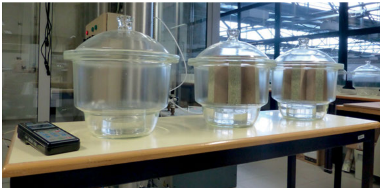
Fig. 8.6: Desiccator method (Japanese standard JIS A 1460).
