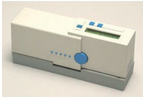
Fig. 1.18: Specular gloss meter/reflectometer.
