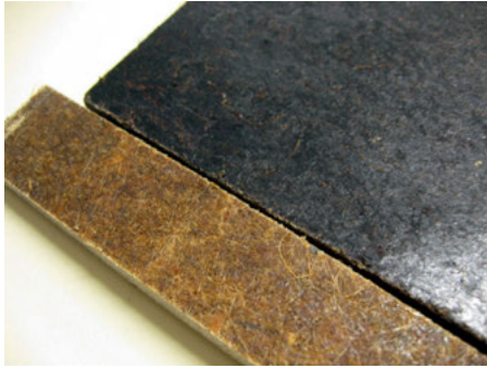
Fig. 3.3: Color difference of a fiber nonwoven mat composite bonded with an epoxide/vegetable oils matrix, lighter colored, and a fiber nonwoven mat composite bonded with a tannin-hexamine system.
