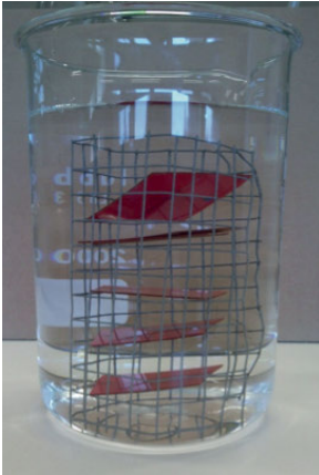
Fig. 1.9: Resistance to immersion in boiling water.
