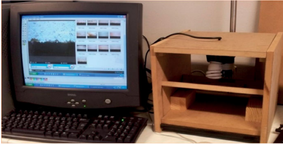
Fig. 8.24: Artificial vision edge quality evaluation system.
