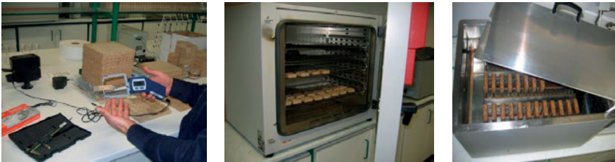
Fig. 8.8: Example of density determination (left), moisture content (center), and thickness swelling (right).
