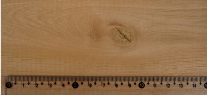
Fig. 7.9: Variation in the size of the feed per tooth measured due to the presence of a wood knot.
