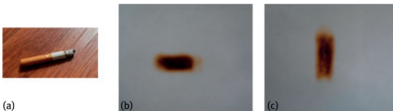
Fig. 1.17: Cigarette test in high-pressure laminates.
