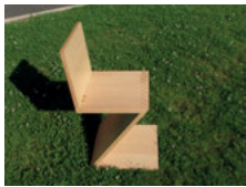
Fig. 6.10: Rietveld minimalist Z-chair built by rotational dowel welding according to the original model.
