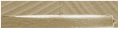
Fig. 6.6: Well-welded dowel where the two pieces to be joined were maintained tightly together by clamping during dowel insertion.
