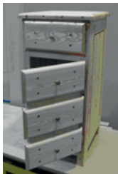
Fig. 6.11: Furniture piece built without any nails, screws or gluing but exclusively by rotational dowel welding.
