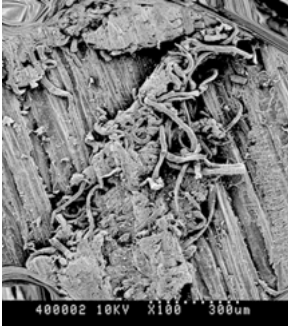
Fig. 6.3: Welded bondline. Note the entangled wood cells (fibers) immersed in a mass of molten material. The whole is superposed on a background of elongated, undamaged wood cells.
