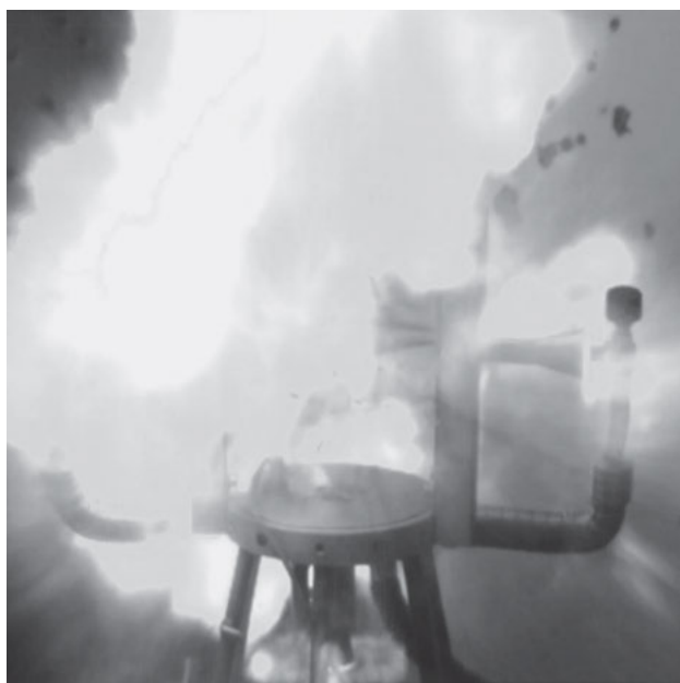
Fig. 9.23: Explosion of bis(trinitroethyl)-1,2,4,5-tetrazine-3,6-diamine (BTAT) in Koenen test.
