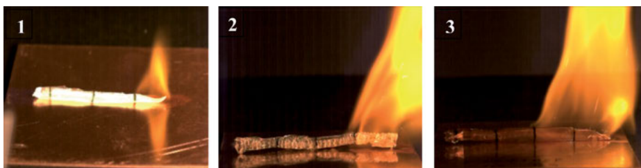
Fig. 2.13d: Burning of three different new formulations of smokeless double-base propellants (from left to right: NC/BTNEO, NC/TNENC and NC/TNEF).
