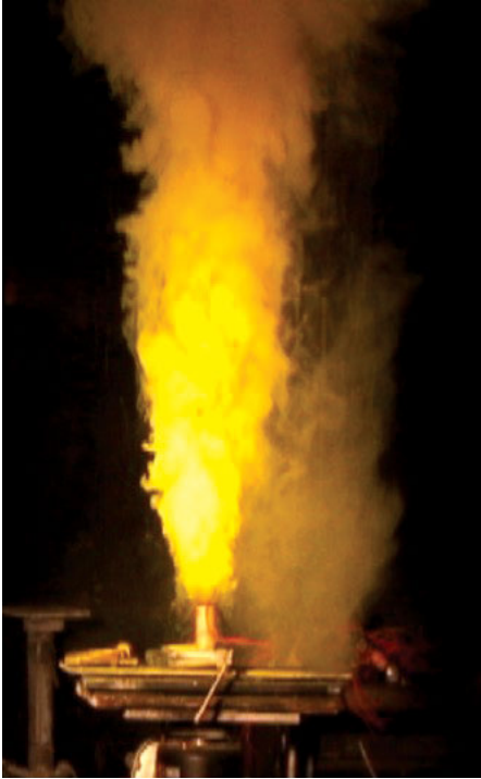
Fig. 2.28b: Image of a smoke fountain generated by the new yellow smoke formulation.
