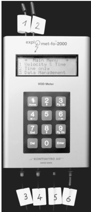
Fig. 7.14: Recording the detonation velocity (VOD, velocity of detonation) using a multichannel analyzer.
