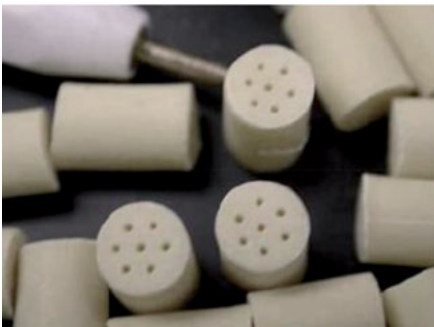
Fig. 4.4b: Solid grain design (top two figures) and actual grains of manufactured HNP (see Tab. 4.11a) with the following parameters: l = 0.055 inches, outer diam = 0.06 inches, inner diam = 0.03 inches, web = 0.016 inches.
