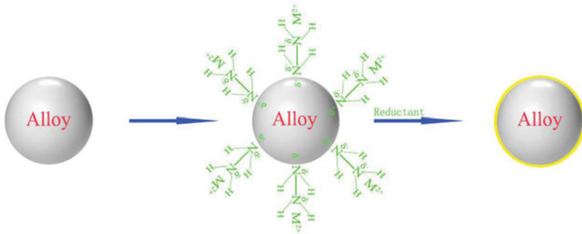
Figure 5.31: Formation of coating layer at alloy surface.
