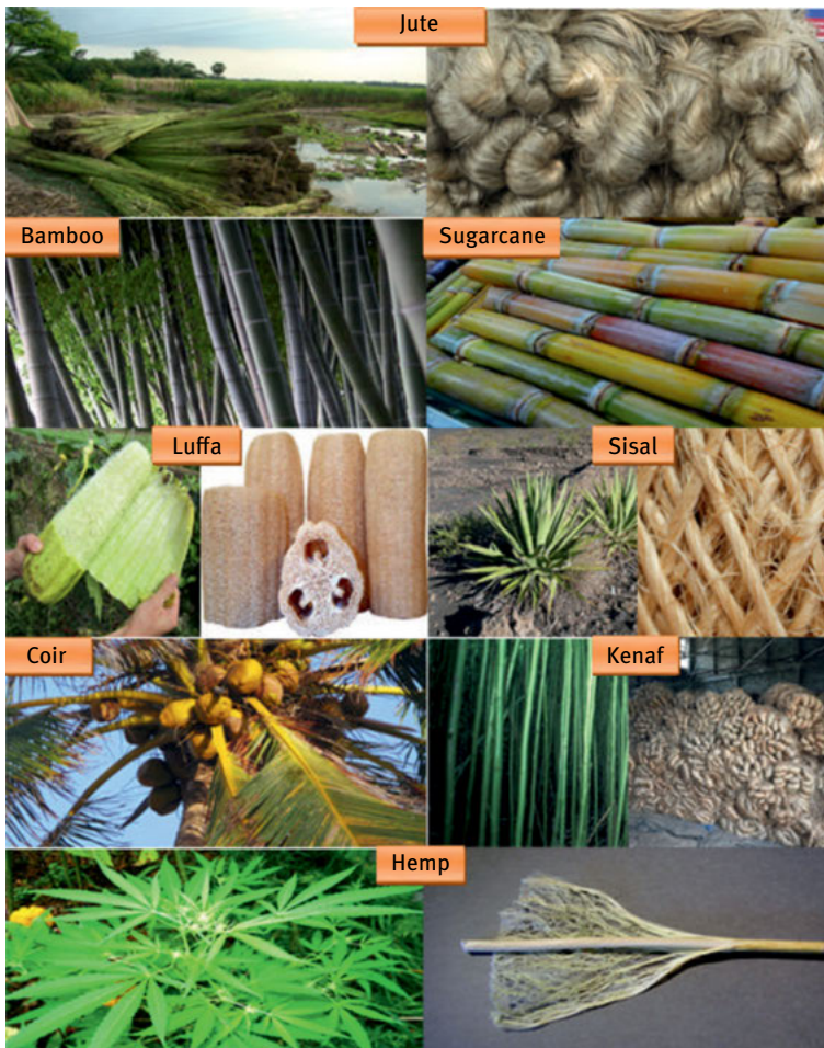
Fig. 2.2: Some commonly used fibers in green composites for engineering applications (source: Wikimedia Commons, Pixabay, Public domain pictures).
