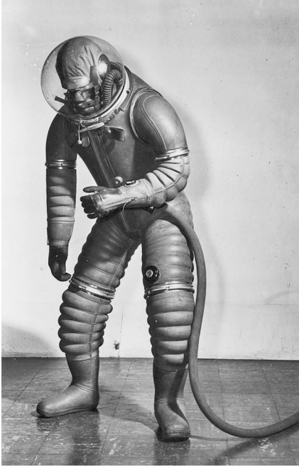
Goodrich pressure suit, circa 1943–50. This World War Two–era pressure suit prototype illustrates the necessity of enabling pilots to function in increasingly austere environments. Photo courtesy of the Smithsonian National Air and Space Museum (NASM USAF-31544AC).
