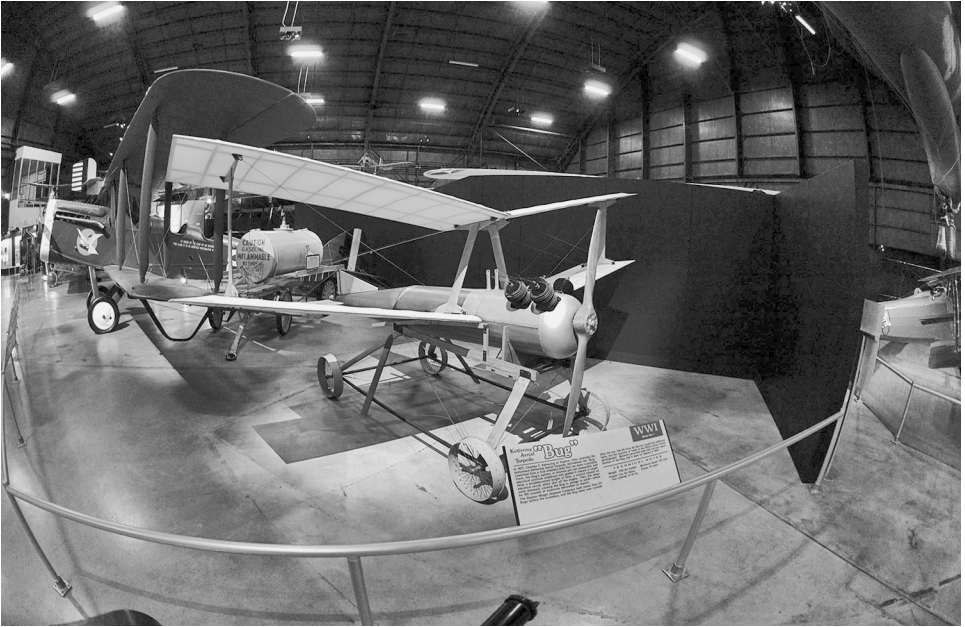
The Kettering Bug. A collaboration of Orville Wright, Elmer Sperry, and Charles Kettering resulted in the Kettering Bug. Flight tested in 1918, it was the Army Air Service's first gyroscopically stabilized unmanned bomber. Photograph courtesy of the National Museum of the US Air Force.
