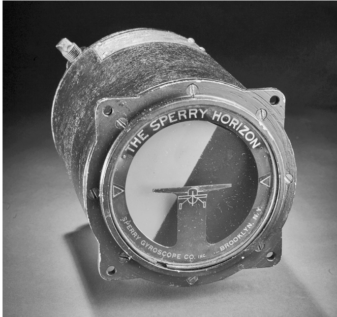
Sperry Gyroscope Company's artificial horizon indicator of the type used by Lieutenant Jimmy Doolittle in the first zero-visibility flight and landing in 1929. This device compensated for the human inability to maintain orientation with the Earth's horizon and fundamentally advanced aviation capability. Photo by Eric Long, Smithsonian National Air and Space Museum (NASM 2014-04796).
