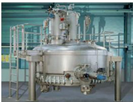
Fig. 5.17: 36 kW (6 generators × 6 kW) batch vacuum dryer for pharmaceutical powder/pellets, Sairem SAS, France
