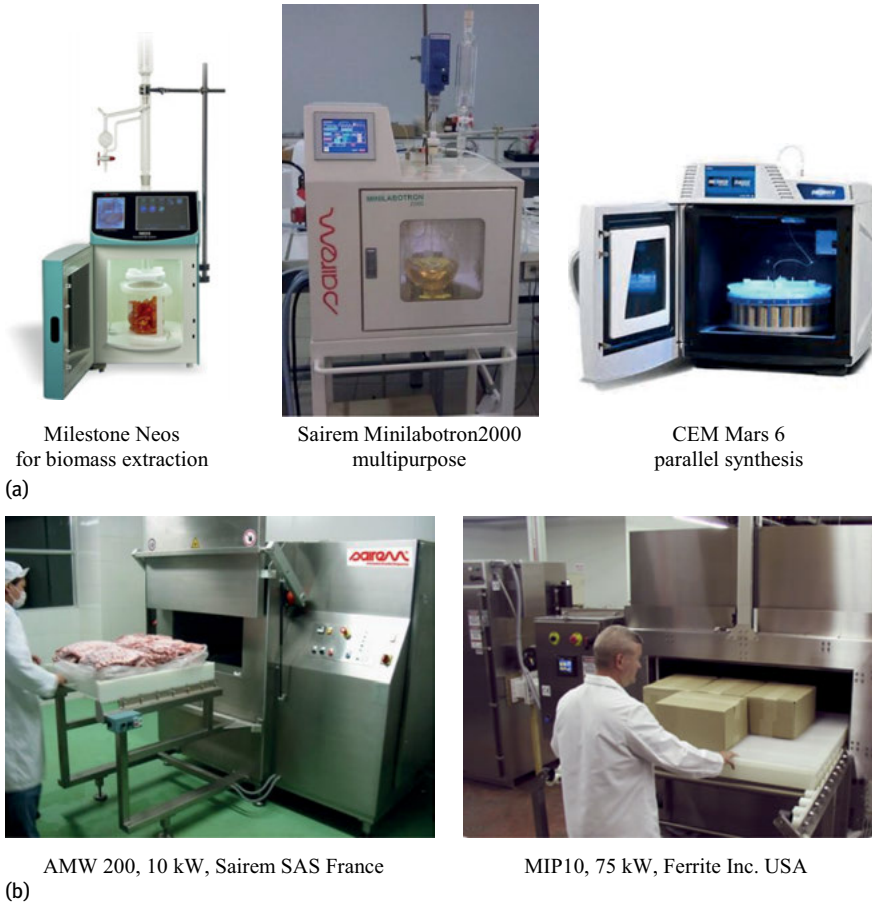
Fig. 5.11: Multimode cavities for laboratory purposes and small production. (a) 2.45 GHz, (b) 915 MHz [8–10, 12]
