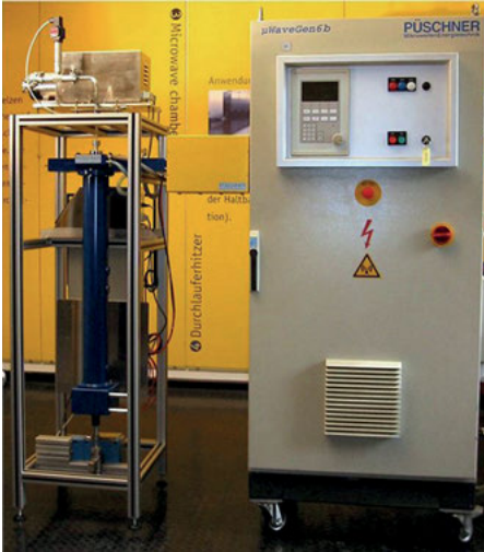
Fig. 5.13: 20 kW (10 generators x2 kW 2.45 GHz CF cooking and pasteurization of liquids, courtesy Puschner, Germany [13]
