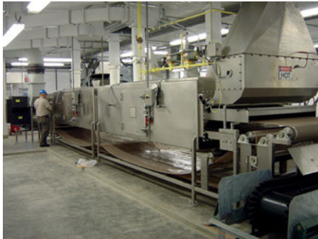
Fig. 5.15: 300 kW (4 generators × 75 kW) 915 MHz, multipurpose continuous-flow dryer, Ferrite, USA
