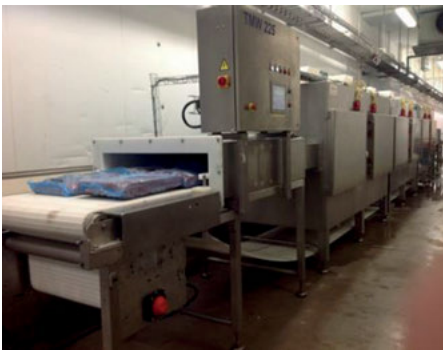
Fig. 5.14: 225 kW (3 generators x75 kW) 915 MHz for meat tempering, courtesy Sairem SAS, France
