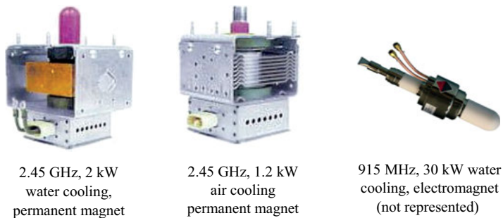
Fig. 5.5: Examples of air and air-/water-cooled magnetrons.
