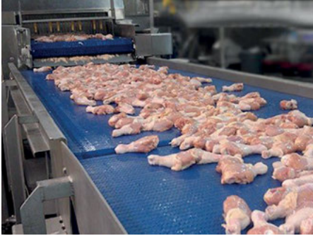
Fig. 5.12: MIP12 – 75 kW, 915 MHz CF preheater (boost heating), courtesy Ferrite Inc. USA [12]
