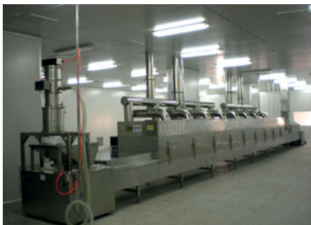
Fig. 5.16: 70 kW, 2.45 GHz continuous flow dryer for chemical powders, Union Microwaves, China [14]
