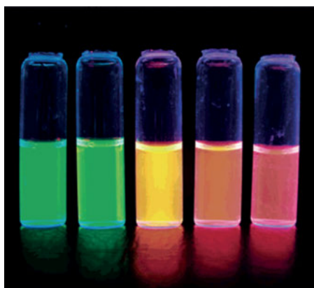
Fig. 14.15: Photograph of wide spectral range of bright luminescence from a sample of microwave-assisted synthesis of CdTe/CdS core-shell nanocolloids in aqueous media without any postpreparative treatment under irradiation with 365 nm UV light from a UV lamp [28]. Copyright 2006 by the American Chemical Society.
