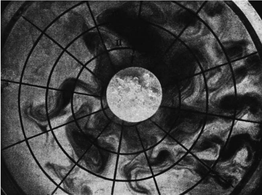
FIGURE 31. Felix Exner's rotating-dishpan model of the general circulation, photographed from above, 1923. Tongues of cold water radiate out from the ice at the center and form vortices akin to cyclones.
