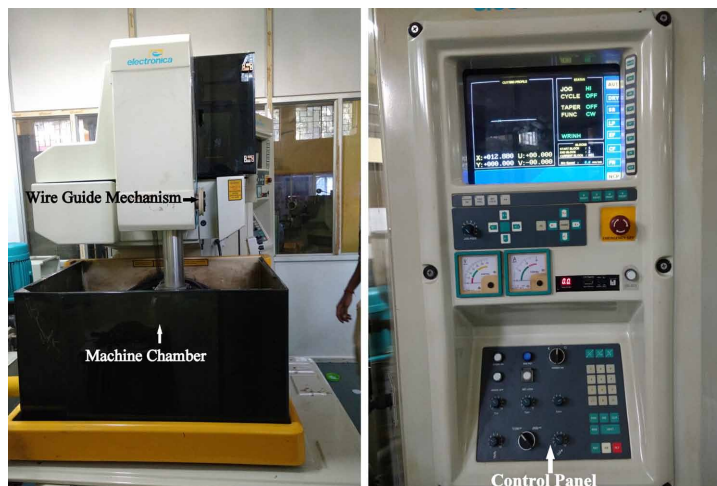
Figure 1. Machining setup of WEDM
