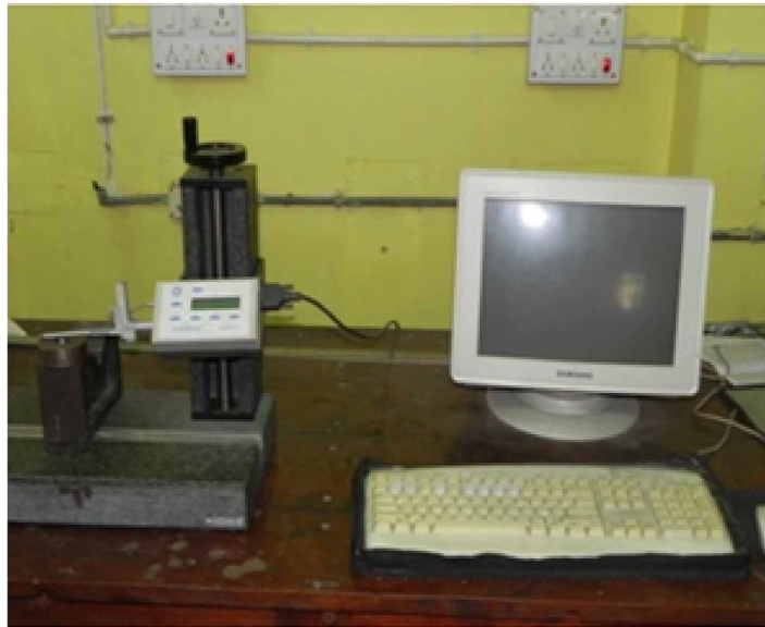
Figure 2. Stylus type profilometer(Talysurf)
