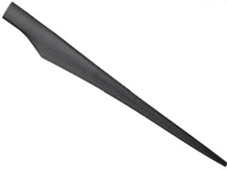
Fig. 9.33: Finite element model of the blade.
