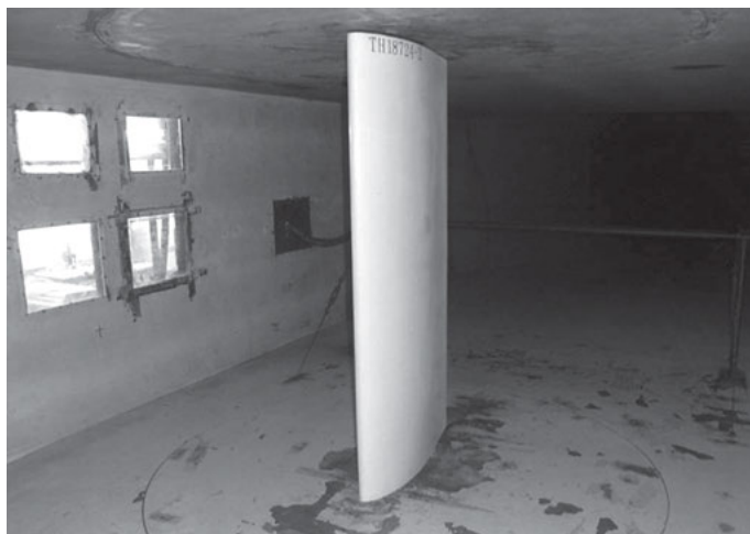
Fig. 5.11: The installation of the model in the wind tunnel (free transition).
