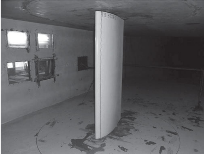
Fig. 5.12: The installation of the model in the wind tunnel (fixed transition).
