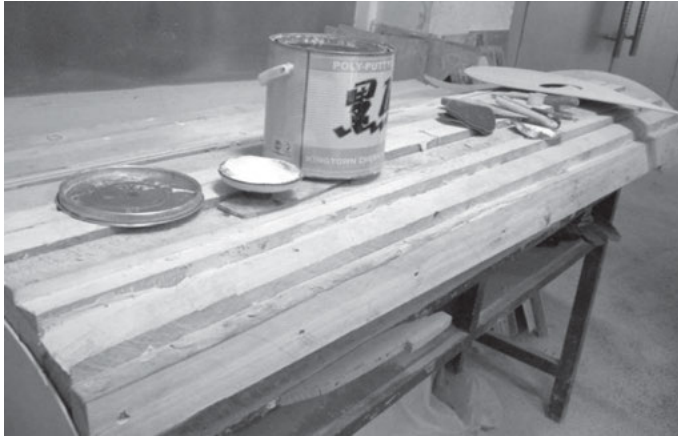
Fig. 5.3: Workblank of the airfoil model.
