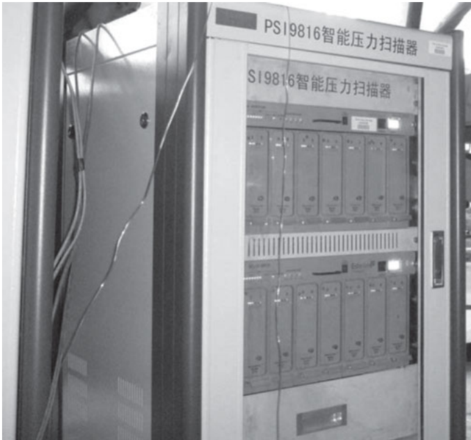
Fig. 5.16: The PSI 9816 pressure data collection system.
