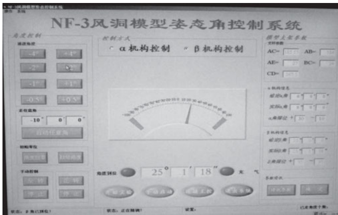
Fig. 5.13: The interface of the AOA control system.
