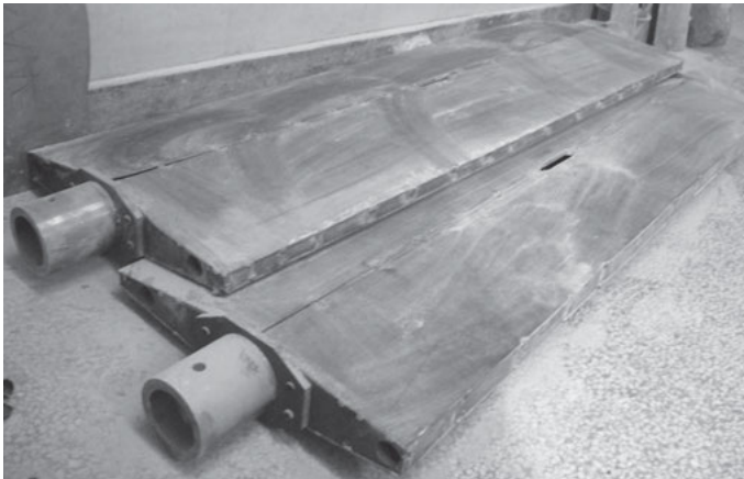
Fig. 5.2: Photo of steel inner structure of the airfoil model.
