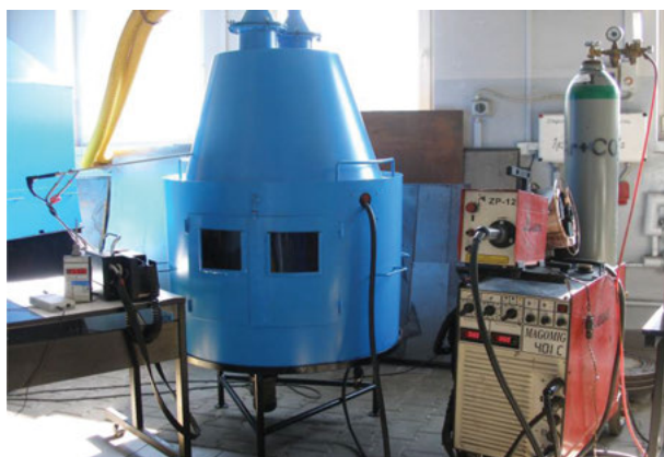
Figure 7.33: Laboratory stand for sampling of dust during MIG/MAG welding of steel [98].
