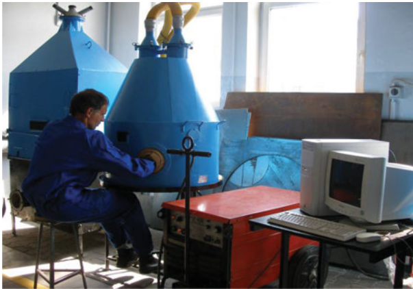
Figure 7.35: Experimental stand for drawing samples of dust generated during MMA welding with covered electrodes [98].
