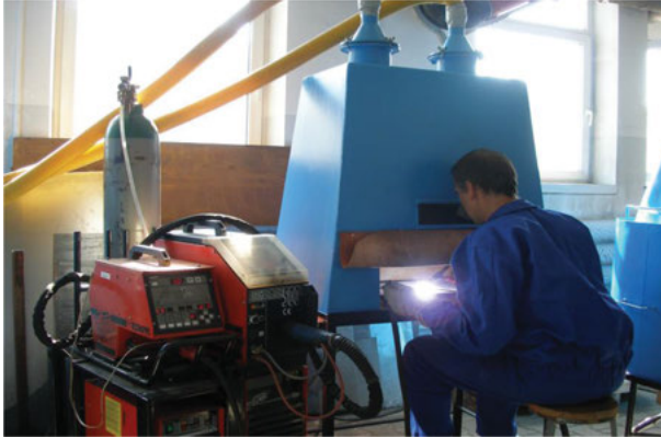
Figure 7.34: Experimental stand for samples drawing of dust emitted while TIG welding of steel [98].
