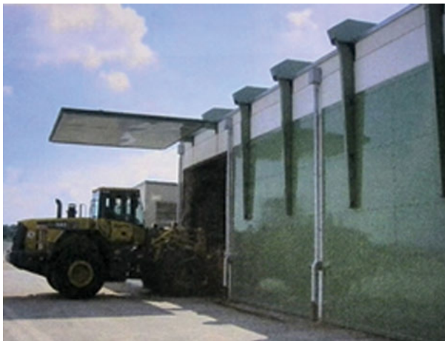
Fig. 4.17: Feeding process of carport dry fermentation.
