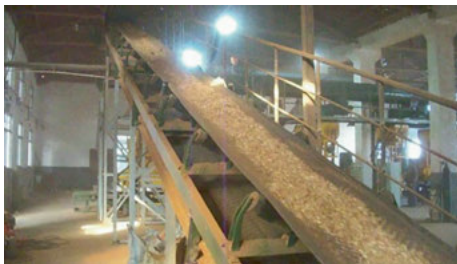
Fig. 5.37: Material supply system.
