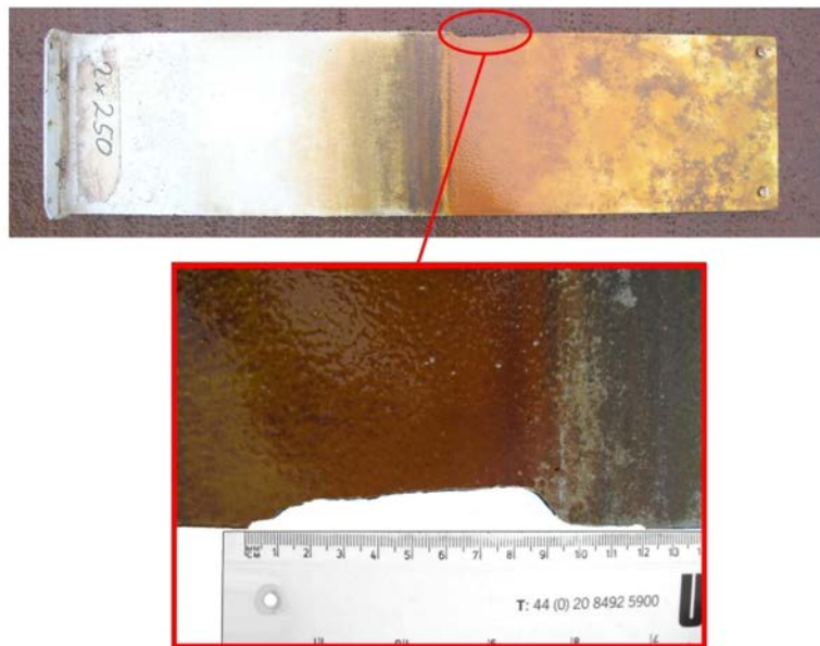
Pitting corrosion at 2-K thick-coat epoxy system at a practically uncoated edge after 138 weeks of instalment in Lake Partwitz
