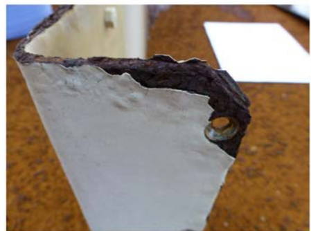
Corrosion on non-standard coated edge - lake Partwitz
