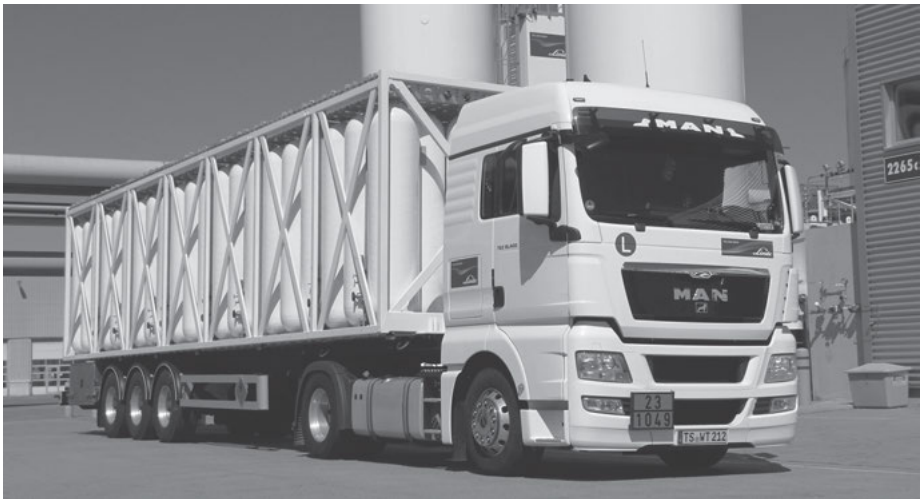
Figure 5.12: Transportation of gaseous hydrogen under 200 bar (Linde Gas).
