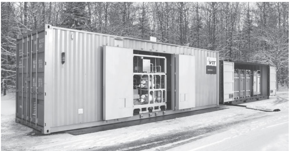
Figure 6.6: Power-to-gas research unit in Finland (VTT Technical Research Centre of Finland Ltd).
