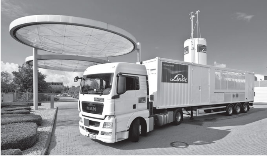
Figure 5.13: Transportation of liquid hydrogen (Linde Gas).
