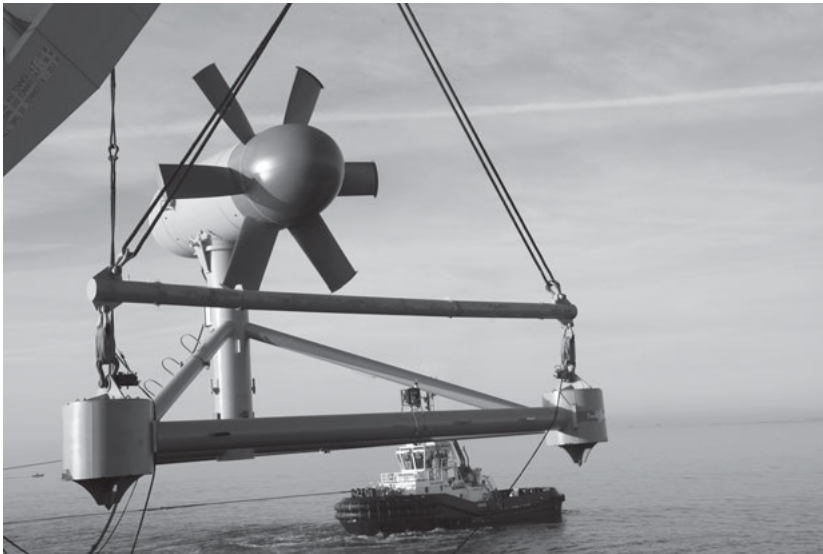
Figure 2.6: Marine current turbine D10 from the French company Sabella.
