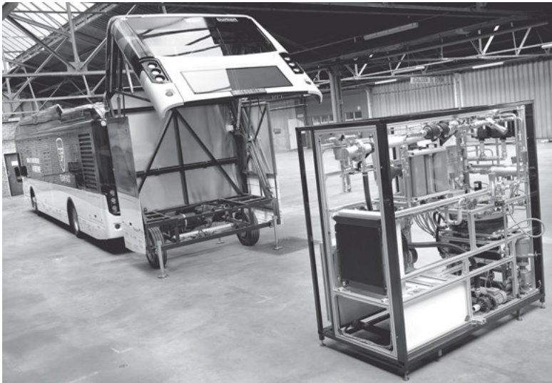
Figure 5.21: Range extender using Hydrozine (TeamFAST).
