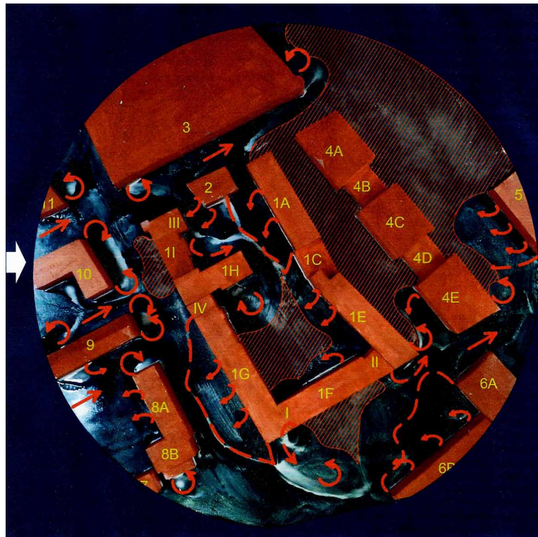
Figure 6. Oil visualization of the improved building development (northern wind) together with airflow markers. The hatching indicates the areas where air exchange is likely to be limited.
