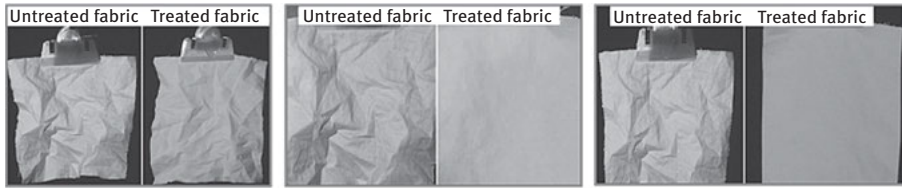
Fabric with wrinkles → Blowing steam on the fabrics → Wrinkle-free effect of the treated fabric
