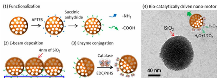
Figure 5. Design and TEM monograph of the biocatalytic Janus mesoporous silica nanoparticles acting as nanomotors. Used with permission from (Ma, X., & Sánchez, S. (2017). Tetrahedron 73, 4883-4886.) Copyright (2017) Elsevier Ltd.
