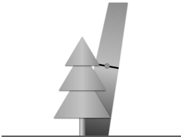
Figure 5. Wide laser beams can produce LIDAR points outside of the tree crown
