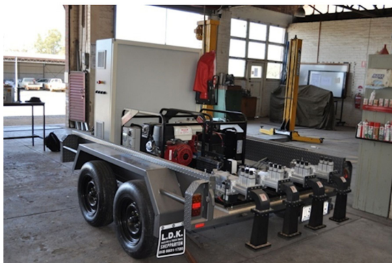
Figure 19.3: Trailer mounted four by 2 kW microwave system to treat weeds and soil.
