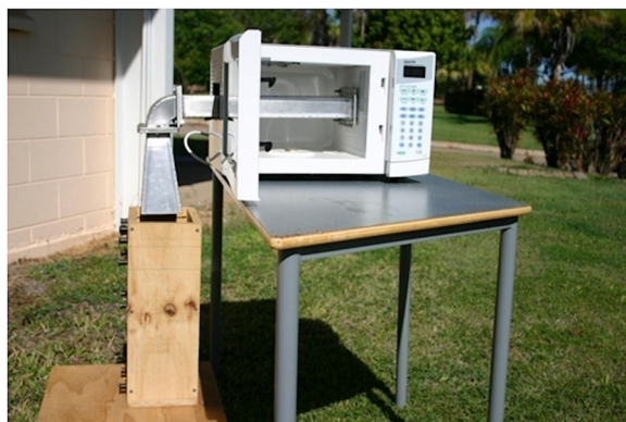
Figure 19.4: Modified microwave oven with a waveguide and horn antenna arrangement to treat weeds and soil (Source: Bebawi, et al. 2007).
