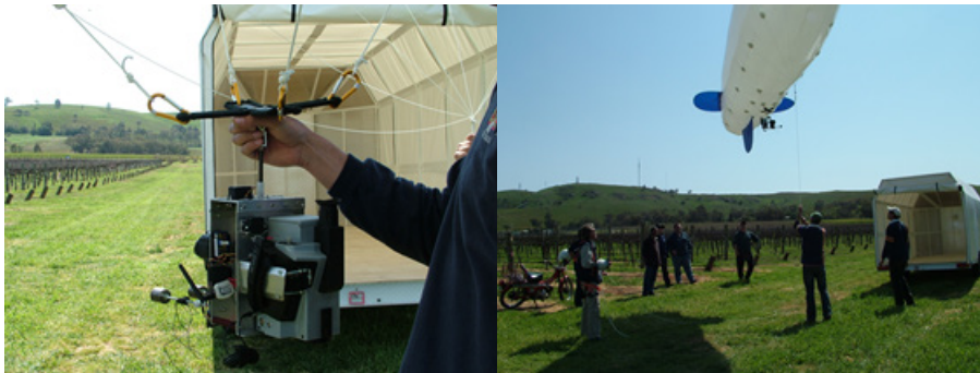
Figure 2.4: (left) Duel camera system with IR and true colour cameras (right) mounted on a transportable airship (Photographs of the system in operation over the vineyard at Dookie campus of the University of Melbourne).
