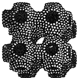
Fig. 2.17: Bicontinuous structure with the surfactant molecules aggregated into connected films characterized by two curvatures of opposite sign [10].
