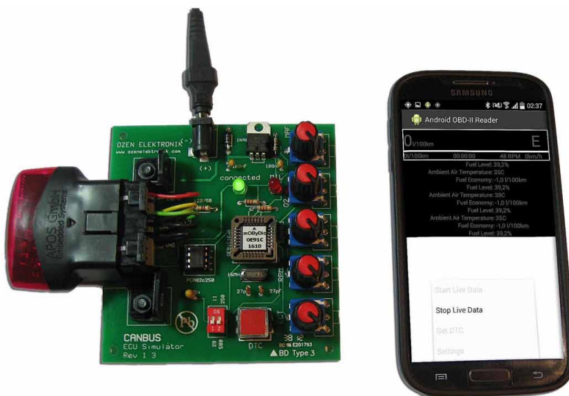
Figure 3. Experimental arrangement for development: OBD-Simulator with connected OBD-Bluetooth-Device and active connection to the smartphone with mobile application “android-OBD-reader”
