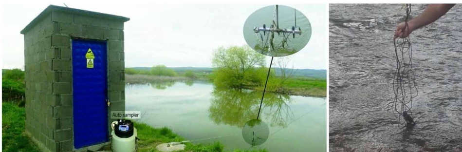
Figure 6. System implementation in Sitnica river – Components: wireless sensor network (also referred to as static sensors) in Plemetin village near the capital Prishtina (middle in the water), auto-sampler (left-bottom), and mobile sensors (right).
