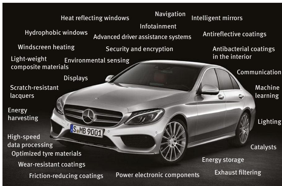
Figure 15.3: Application fields of nanotechnology for automobiles, based on [8].
