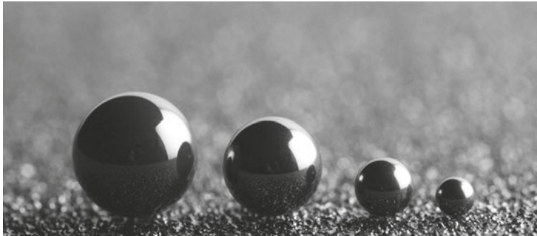
Figure 17.19: Diamond spheres of different diameters after CMP processing. The diameter ranges actually from 0.6–8 mm. It is expected that larger and smaller diameters can be produced in the near future.
