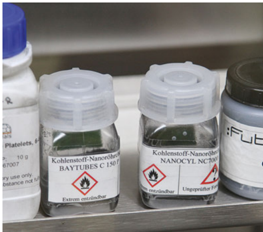
Figure 18.7: Example for a simplified labelling of a storage bottle with pictogram and short phrase.
