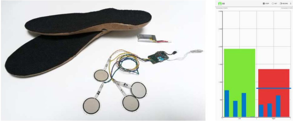
Figure 1 Left: The multimodal biometric measurement system for mobile gait analysis and therapy monitoring, eSHOE. The embedded electronic components can be seen besides the insoles. Right: Screenshot of the smartphone biofeedback application while the load applied on the right foot is monitored, the load being applied has exceeded the predefined threshold value (blue horizontal line).
