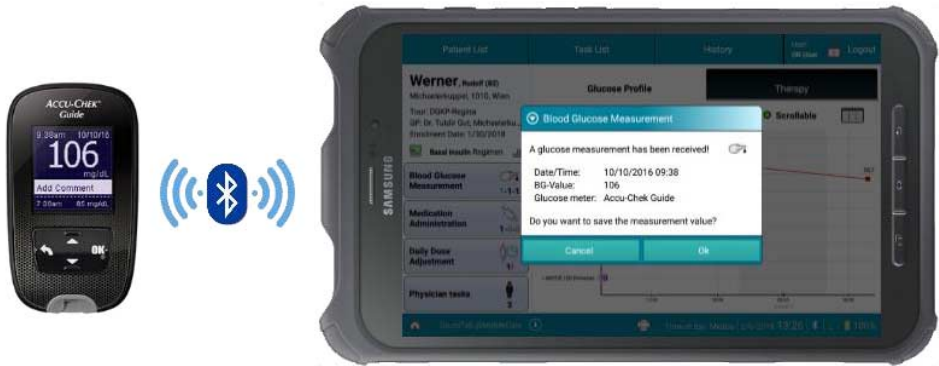
Figure 1. Transmission from Accu-Chek® Guide glucose meter to GlucoTab® CDSS.
