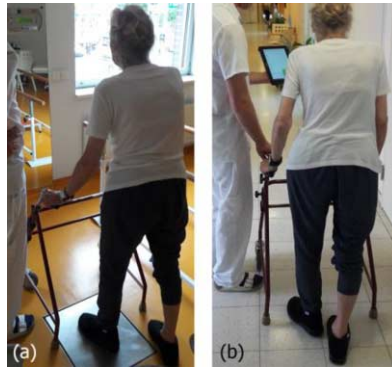
Figure 2: (a) The calibration process of the biofeedback system using a force plate. (b) Patient becoming visual feedback during a measurement.
