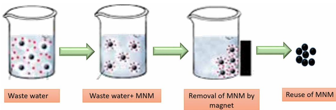
Figure 2. Schematic representation of use of MNM and their removal from wastewater
