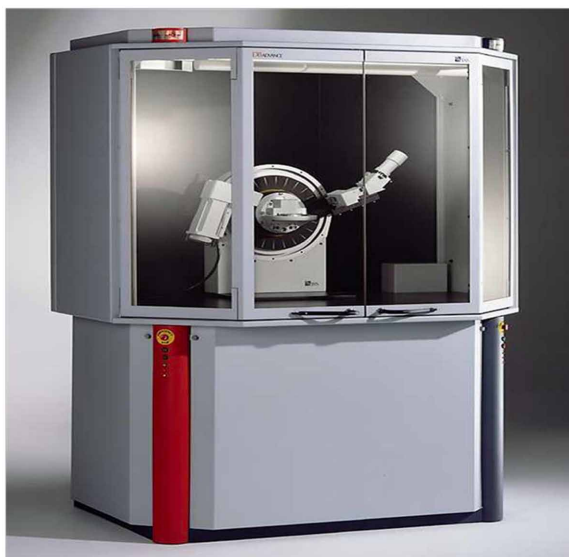
Figure 5. A PXRD (Bruker D8 Advance) showing the goniometer and its drives inside the cabinet (Chauhan & Chauhan, 2014)
