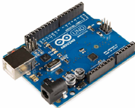
Figure 3. Arduino UNO Microcontroller Development Board
