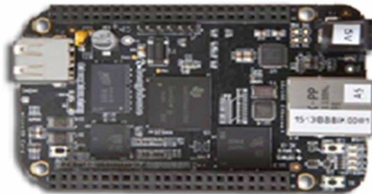
Figure 5. BeagleBoard-Single Board Computer
