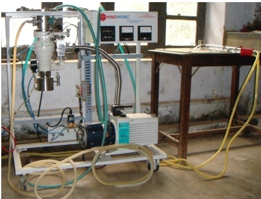
Figure 3.1 Vacuum pumping system used to evacuate the quartz tubes containing the samples (Hind Hivac Make; Model VS – 65D; 10^{-6} Torr).
