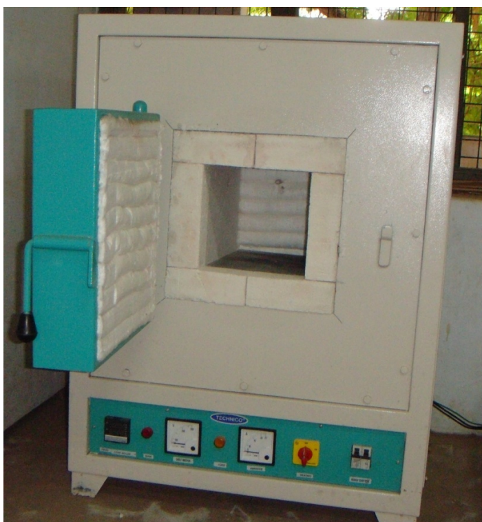
Figure 3.2 Microprocessor controlled high temperature furnace used for melt growth of the DMS samples (Technico Make; Max. temp: 1200^{\circ}\text{C} ).
