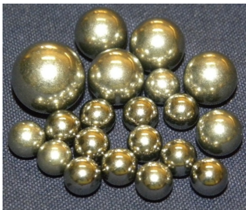
Figure 3.7 Milling media (Stainless steel balls) used to grind the elemental powders.
