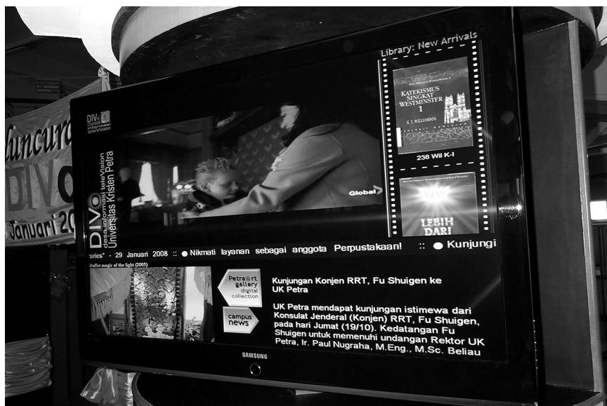
Figure 6.1. Pilot phase of the Divo project. The screen was divided into seven different zones including an upper zone with elements of (left to right): static image, video, and scrolling images plus text; a middle zone with ticker text; and a lower zone with elements of (left to right): dynamic images from institutional repository, static image, and scrolling text. Photographer: Toong Tjiek Liauw
