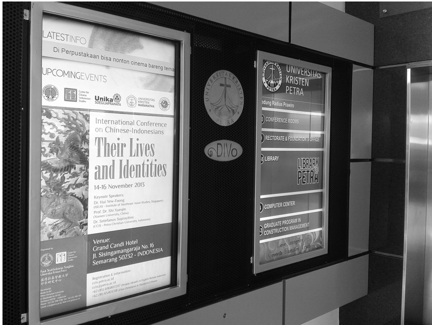
Figure 6.2. Wall-mounted unit of DVo 3.0, installed beside the elevator of W Building. The screen on the left is a DS screen, and the one on the right is an analog or print-based backlight poster of the building directory, which can be converted into another DVo screen if needed. Photographer: Toong Tjiek Liauw
