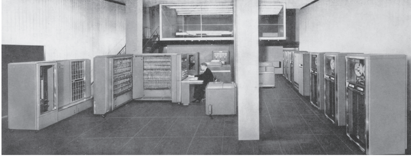
FIGURE 6.1. The IBM 704, ca. 1954. Your laptop is about 250,000 times faster than this machine and has about 100,000 times as much random-access memory. (Source: IBM 704 Manual of Operation , 1954.)
