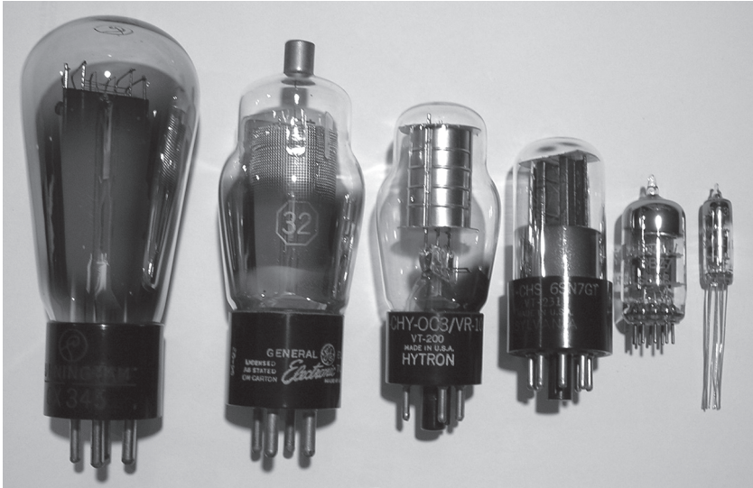
FIGURE 3.3. Life before the transistor: six vacuum tubes, representative of the 1920s through the 1960s. From left to right: Cunningham CX345, 32 (GE), VR-105 (Hytron, also OC3-A), 6SN7 (Sylvania), 6BQ7A/6BZ7/6BS8 (RCA), 5636 (Sylvania, imprinted “Engineering Sample,” a subminiature). The Cunningham is 5\frac{1}{8} inches top to bottom. (From the author’s garage.)
