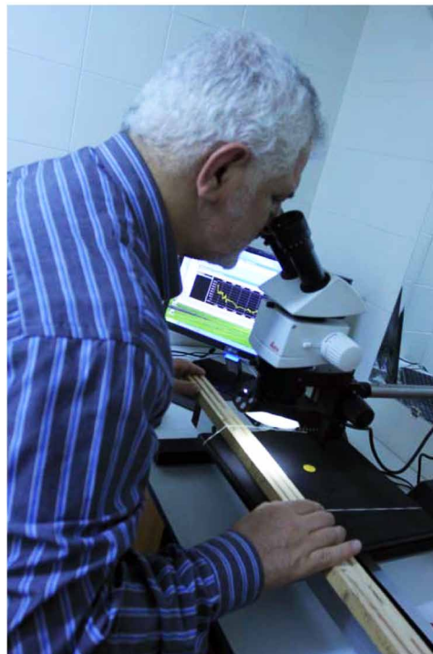
Figure 6. Measuring core sample tree ring widths in the dendrochronology lab. using computer equipped machine (Author, 2012)
