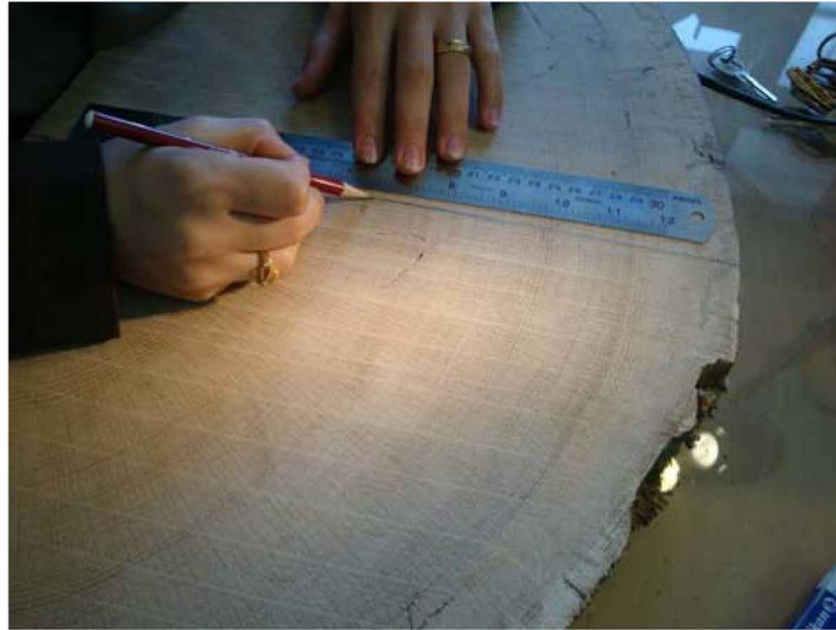
Figure 5. Measuring disc sample tree ring widths in the Golestan research centre lab. using manual measurements (Author, 2010)
