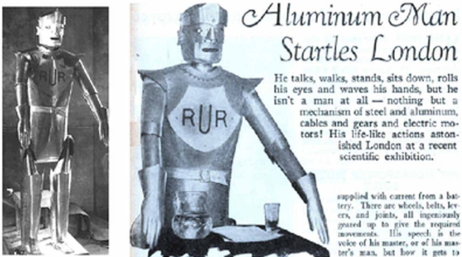
Figure 9. Robot named Eric RUR (RUR comes from Carel Capek's play RUR – Rossum's Universal Robot, where the term robot was coined) – the robot photograph and the title page of the article /Chronicle Telegram 26 Nov 1928/.
