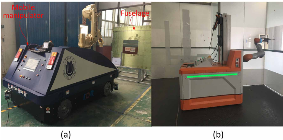
Figure 20. Mobile manipulator for aerospace manufacturing (a) and for decoration engineering (b)
