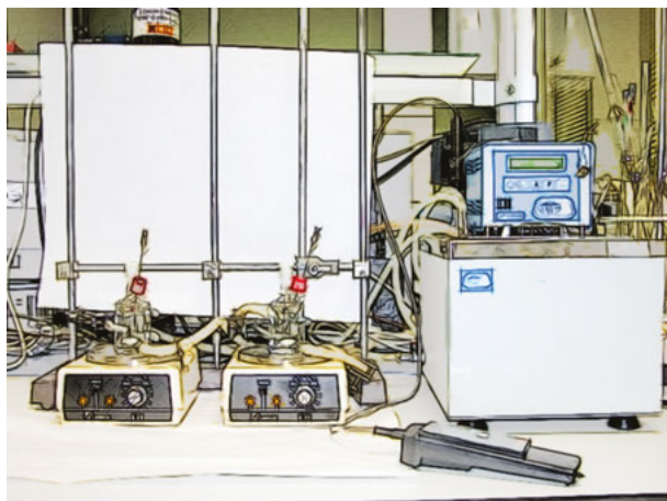
Figure 3.3: Equipment commonly used in the measurement of solubilities of amino acids at atmospheric pressure: thermostated cells with agitation device.
