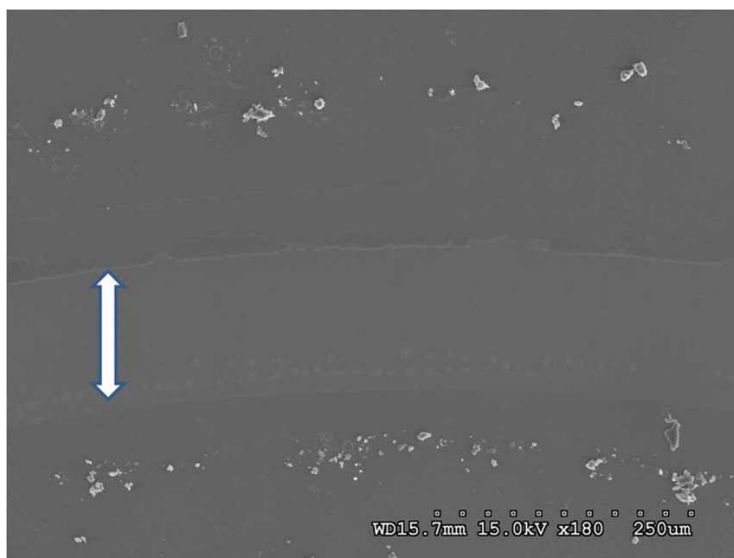
Figure 2. Worn surface of silicon tested at micro-scale. At micro-scale, silicon undergoes wear within a short duration of time, i.e. it has low durability
