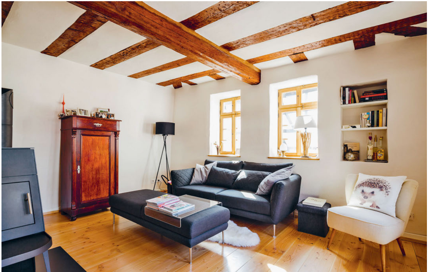
The floors were laid with solid Douglas fir planks with a vapor-permeable finish, supporting a great indoor climate due to their humidity-regulating properties.
