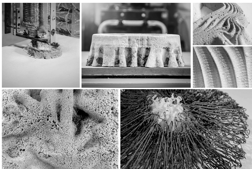
Figure 4.4 C-Biom.A group/IAAC – BiotA Lab/Bartlett UCL, material research, 2015–16. Upper row (left): In:Sand:Out – robotic printing with sulphur concrete. Project: Kunaljit Singh Chadha; Supervision: Professor Marcos Cruz Upper row (right): Design for ageing building – cactus mucilage mortar casts. Project: Yessica Mendez; Supervision: Prof Marcos Cruz Lower row (left): Pervious branching – moss seeding on bioreceptive brick. Project: Chang Lui, Zhixiong Yang, Chae Ah Ahn; Supervision: Professor Marcos Cruz, Richard Beckett, Javier Ruiz Lower row (right): Filatures – prototype of façade screen with mycelium growth. Project: You Han Hu, Cheng-Hsiang Lew, Yuan Jiang, Xia Chen Wei; Supervision: Professor Marcos Cruz, Richard Beckett, Javier Ruiz
