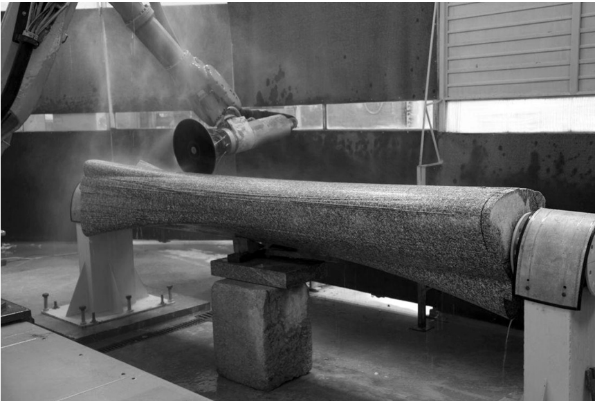
Figure 2.10 A combination of seven axes of movement allows the robot-borne cutter to produce columns over 6 metres in length from a single piece of granite.
