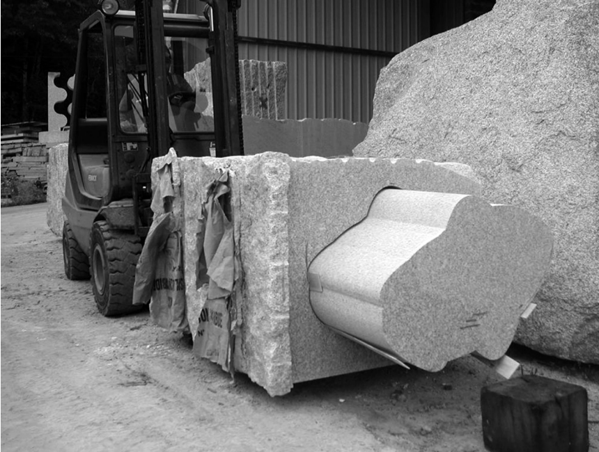
Figure 2.9 In order to give the robot the least amount of work to do, a diamond-encrusted wire cuts the smallest possible blank for the robot to work on.
