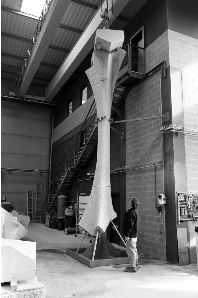
Figure 2.11 A completed column, cut entirely by robot-borne saws, over 9 metres in height.
